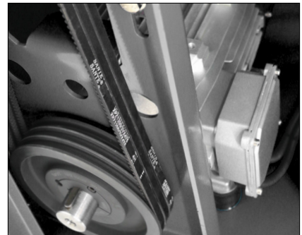
Pulley-belt transmission and IE3 electric motor
